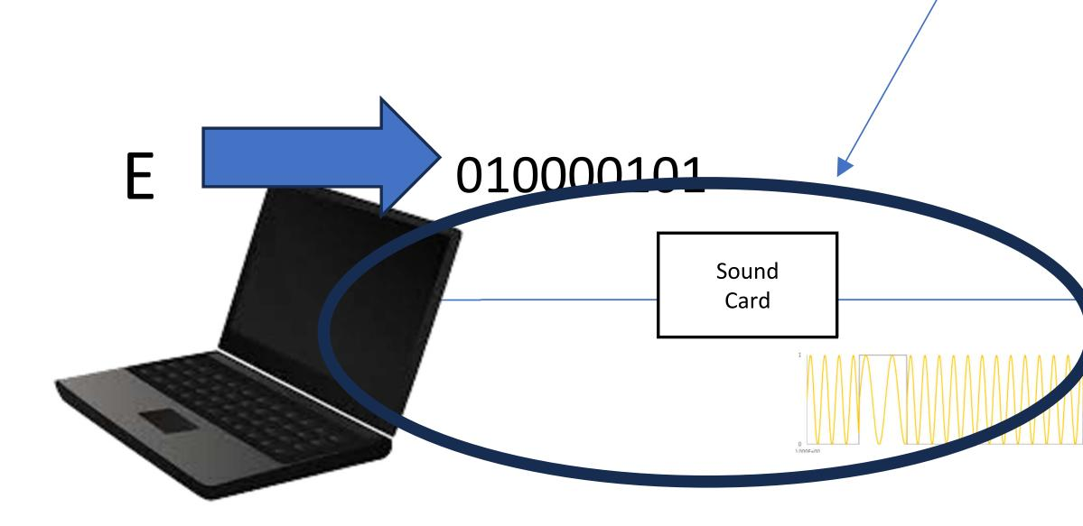
A Terminal Node Controller TNC that is split between software on a personal computer and a sound card.
